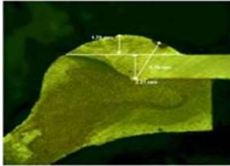
Zone 3 Weld (Microscopic view)
